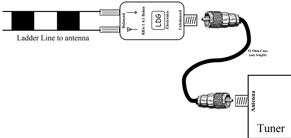
A note about ladder line: unlike coax, ladder line performance can be strongly influenced by conductive elements nearby, such as aluminum house siding, gutters, other wires or the earth. You must take care to route your ladder line correctly, using standoffs and insulators as needed. To avoid a degradation of performance, mount your balun remotely and use coaxial cable to connect to the tuner or radio.
